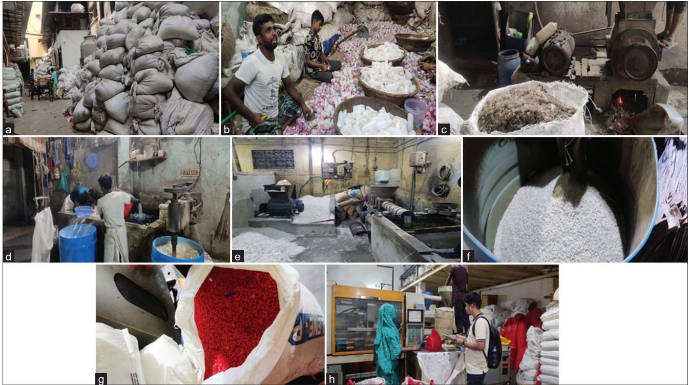
Figure 4: Plastic waste recycling cycle. (a) Collection of plastic. (b) Sorting and segregation. (c) Shredded by a crushing machine. (d) Washing. (e) Pelletize production by cutter machine. (f) White granules. (g) Reproduction plastic. (h) Final product (plastic belcha, bucket, etc.)
