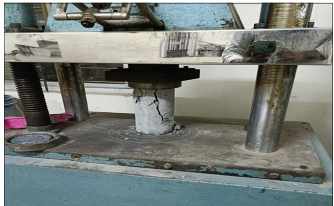
Figure 2: Compressive strength test
