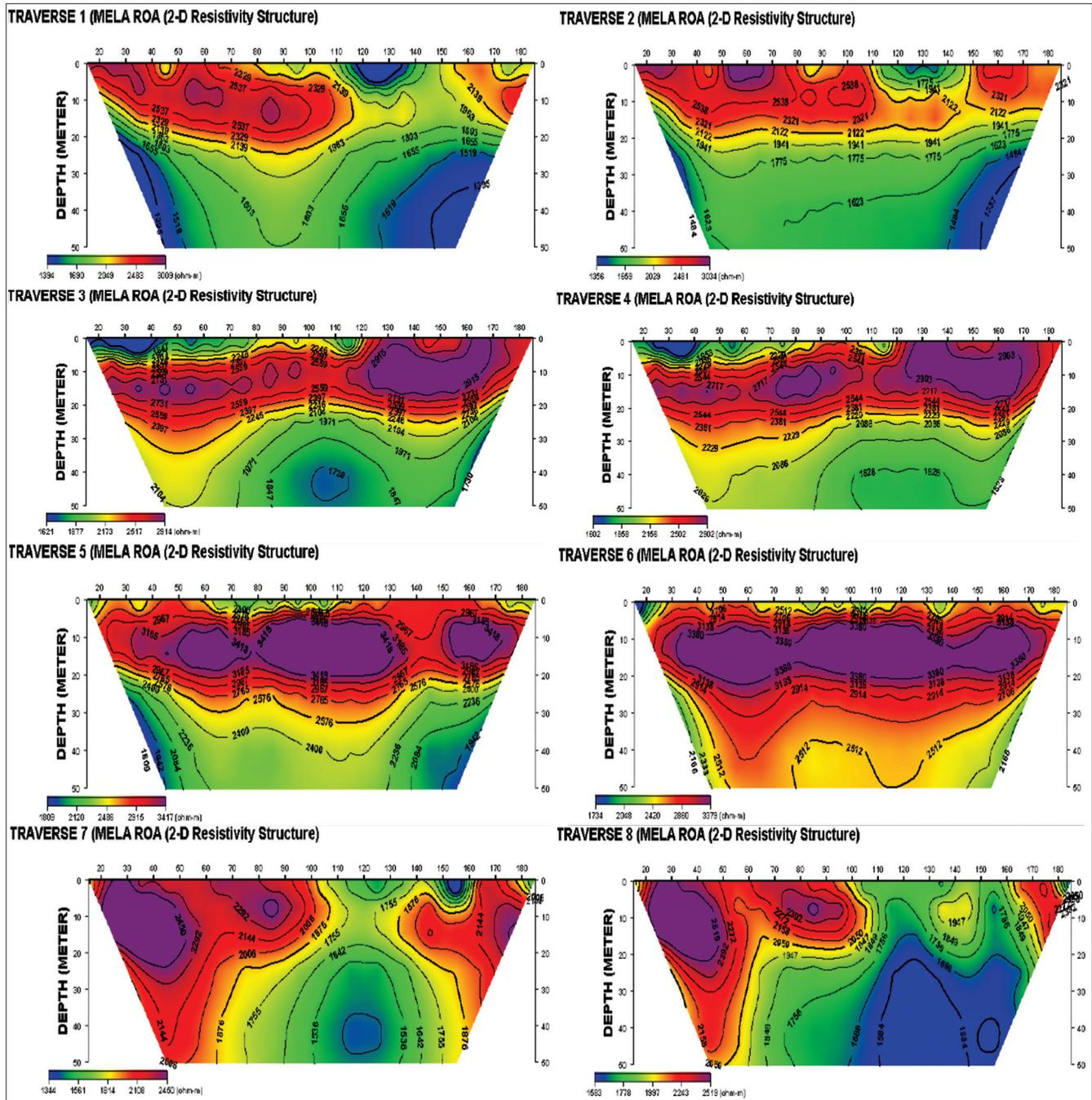
Figure 3: 2D electrical resistivity imaging sections along traverse 1–8
