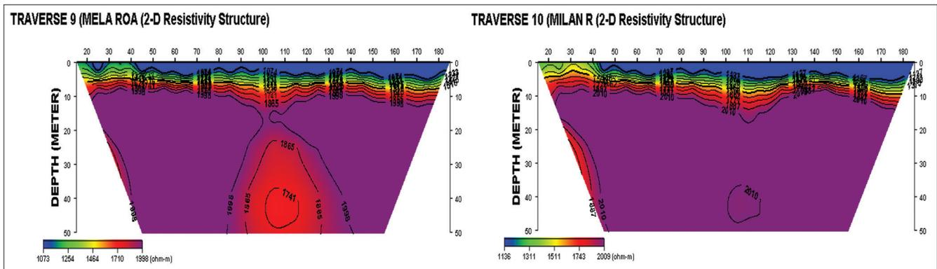
Figure 4: 2D electrical resistivity imaging sections along traverse 9–10
