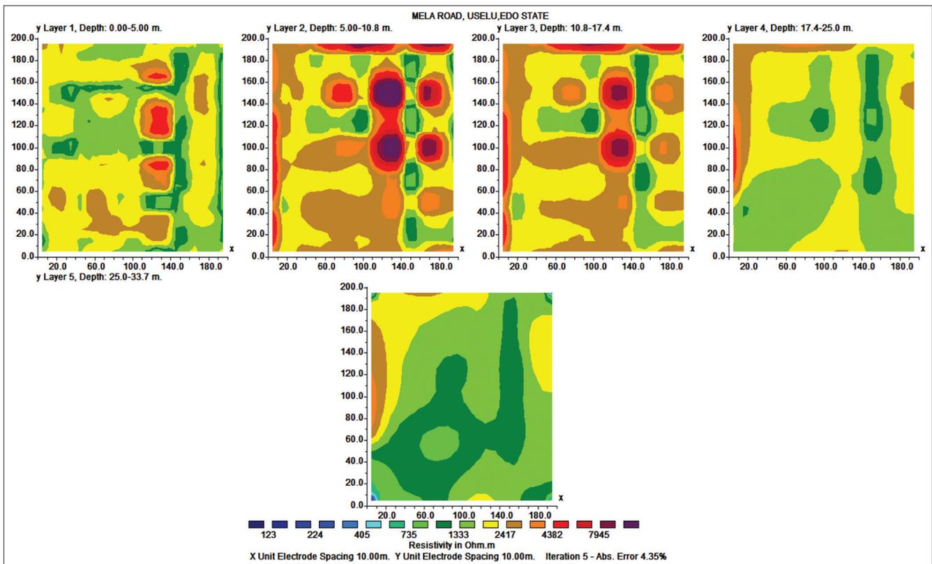
Figure 5: Horizontal depth slices obtained from the 3D inversion of square 2D profiles
