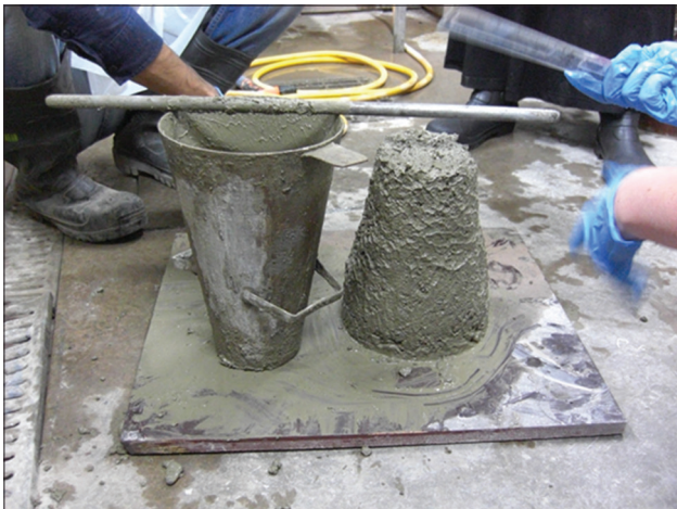
Figure 1: Slump measuring and testing
