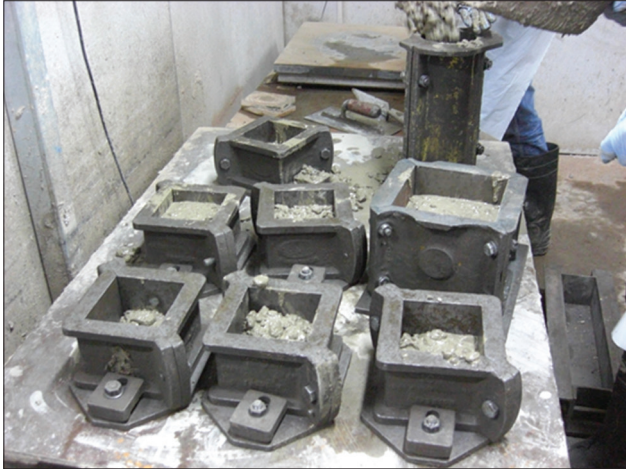
Figure 2: The picture shows the casting of concrete for testing specimens
